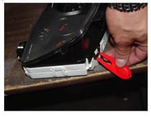
Step 9. While wearing supplied gloves, peel off sticker back of the new gauge face and apply to cluster.
