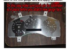
Step 12. Once all the needles are on turn the vehilce off then start again. Make sure they are properly positioned, and push down just alittle.
