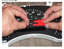
Step 10. Once the gauge face is on, plug instrument cluster back in, and start vehicle.
