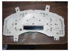
Step 11. With the vehicle running, In reference to the sketch you made in step 1, Lightly push on the needles where they were pointing.
