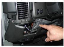
Step 5. Remove the four 7mm screws holding the instrument cluster in place, and unplug...
